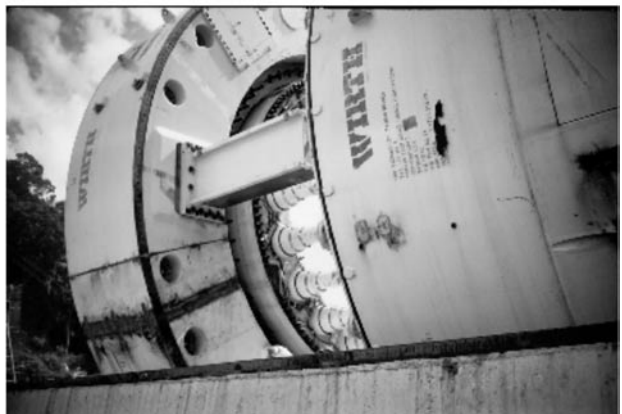
Figure 11. Connect the cutter head shield and gripper shield.
